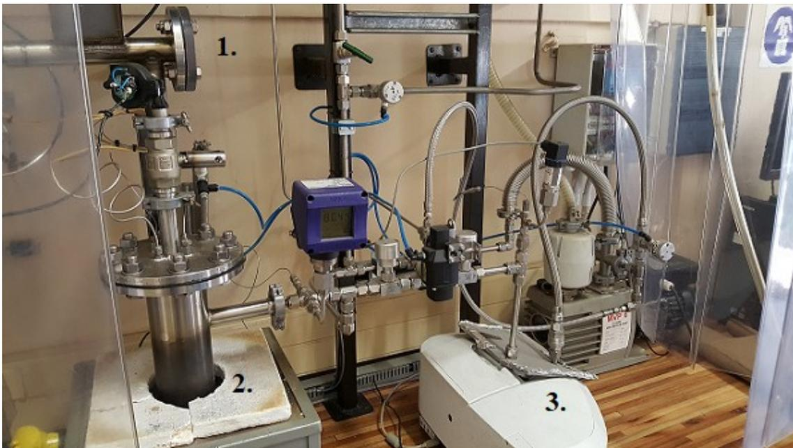
Figure 3: Pyrolysis setup at the University of Pretoria, Fluoro-Polymer Laboratory indicating pyrolysis reactor and Perkin Elmer Spectrum Two FTIR
